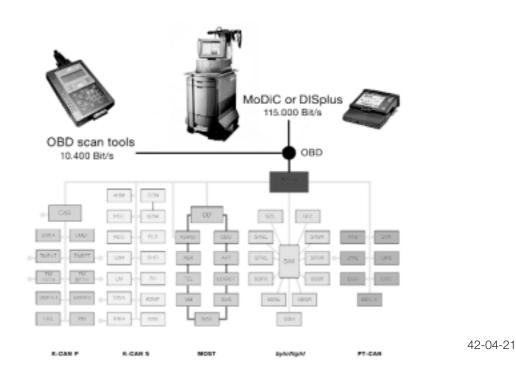
The ECM is not directly connected to the OBD diagnostic connector. The OBD diagnostic connector is connected to the ZGM. The ECM is connected to the ZGM (central gateway module) by the PT CAN bus. The ECM is also connected to the Valvetronic control module by the Lo CAN (local) bus. Valvetronic faults are stored in the ECM.
